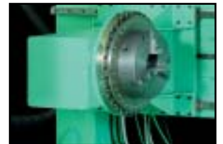
Welding head Robust - incorporates our unique 4-wheel wire feed system
