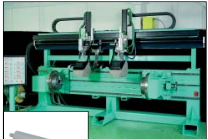
Multi Surfacers R 3000 for cladding rolls (built with two welding heads)
