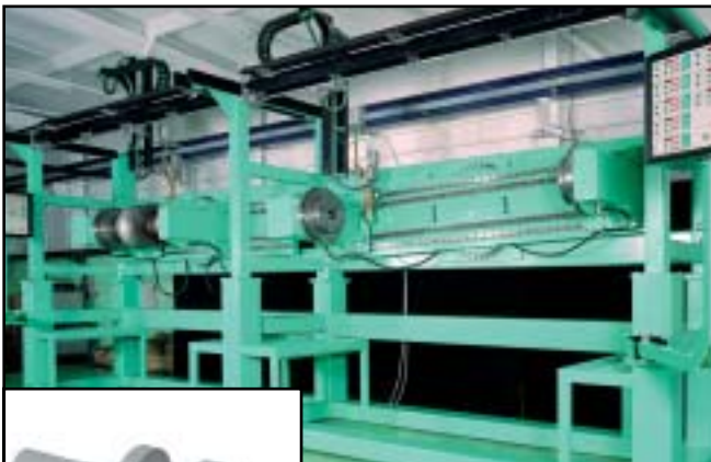
Multi Surfacers PFR 1 for cladding pipe forming rolls from the steel industry (built as a twin workstation)
