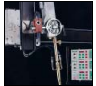
Welding head Robust - incorporates our unique 4-wheel wire feed system
