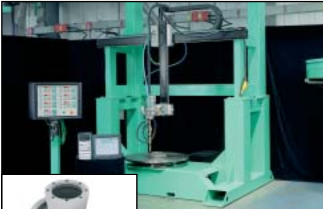
Multi Surfacers ID 1000 for cladding valves from the petro chemical industry
