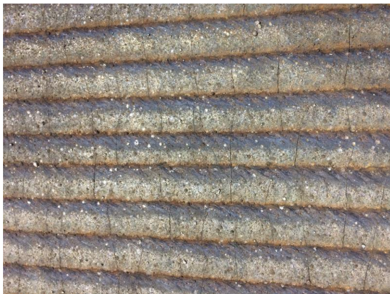
Fig. 2: Hardfaced Plate with Chrome-Carbide-Matrix.
