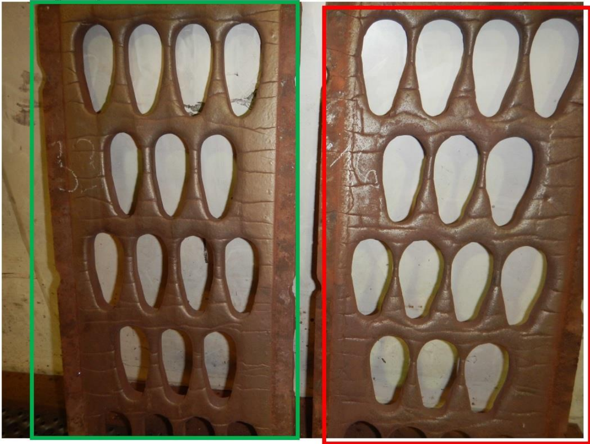
Fig. 4: Comparison: Advanced Plates (left/green/30weeks) <-> Standard Plates (right/red/weeks).
